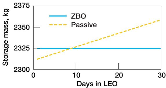
Figure 4.—Passive and ZBO cryogenic thermal storage mass versus duration for LCH<sub>4</sub> storage in 2.2-m-diam tank.
