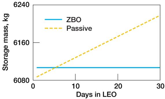
Figure 3.—Passive and ZBO cryogenic thermal storage mass versus duration for LO<sub>2</sub> storage in 2.2-m-diam tank.
