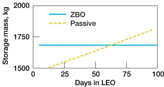
Figure 5.—Passive and ZBO cryogenic thermal storage mass versus duration for LH<sub>2</sub> storage in 3.3-m-diam tank.
