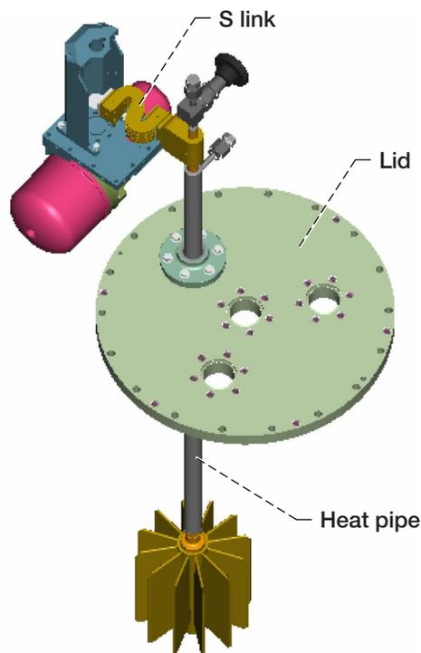
Figure 2.—Integration design connects cryocooler to propellant tank lid.
